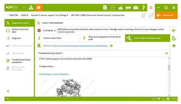
New repair **SMART guides** by fault code in the **JOHN DEERE LEVEL 40** engine control system, present in several models of tractor and harvest equipment.
