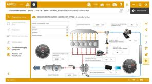
**EMR5 EDC MD1** (*on SAE J1939*) engine control system, System Display, activations, system checks and maintenance service operations.
